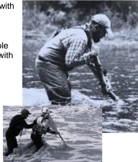
Figure W65. Tripod position for a shallow water crossing.
