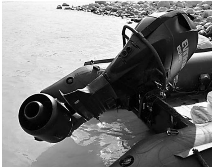
FIGURE W48. Evinrude 55-hp two-stroke multi-fuel outboard engine with a shrouded impeller, which handles submerged obstacles and is safe to operate around swimmers.
