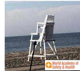
Lifeguard chair for a single lifeguard. It is elevated above the level of the swimmers and far enough behind the high tide line that it is not washed away or damaged by the incoming tidal flow and/or wave action.
