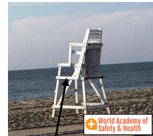
Lifeguard chair for a single lifeguard. It is elevated above the level of the swimmers and far enough behind the high tide line that it is not washed away or damaged by the incoming tidal flow and/or wave action. FIGURE C.7.3
